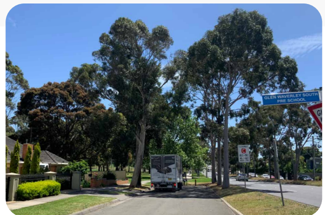
Canopy trees provided along service road, where verge and outer separator are of sufficient width.
